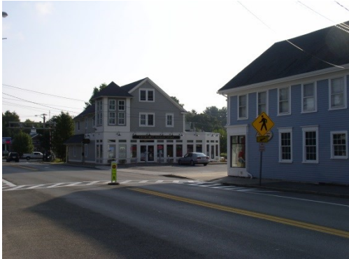
● Figure 13: Example of building design using trim boards, roof dormers, large expanses of glass on the pedestrian level, interesting roof line and a contemporary expression.
