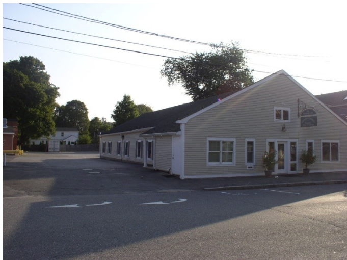
● Figure 8: Example of inappropriate design with scale and proportions of trim, roof line, entry door and building height to width.
