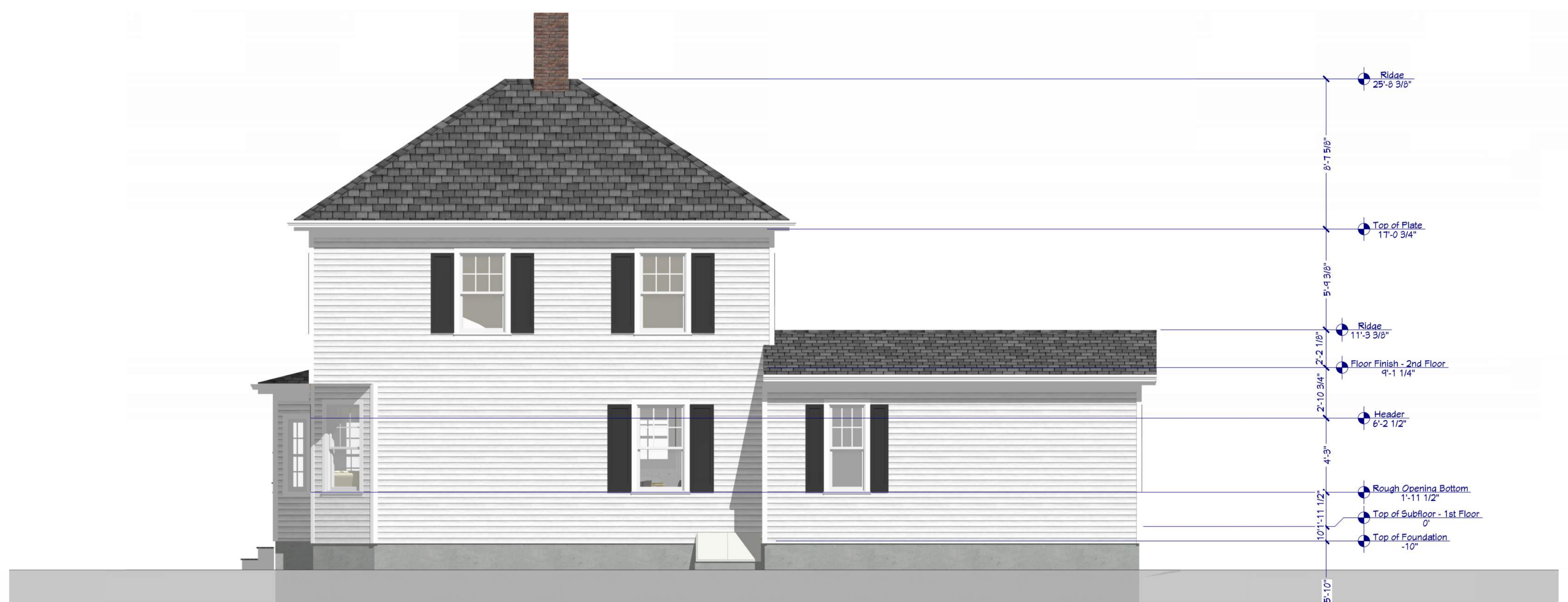
Exterior Elevation Right 1/4 in = 1 ft
