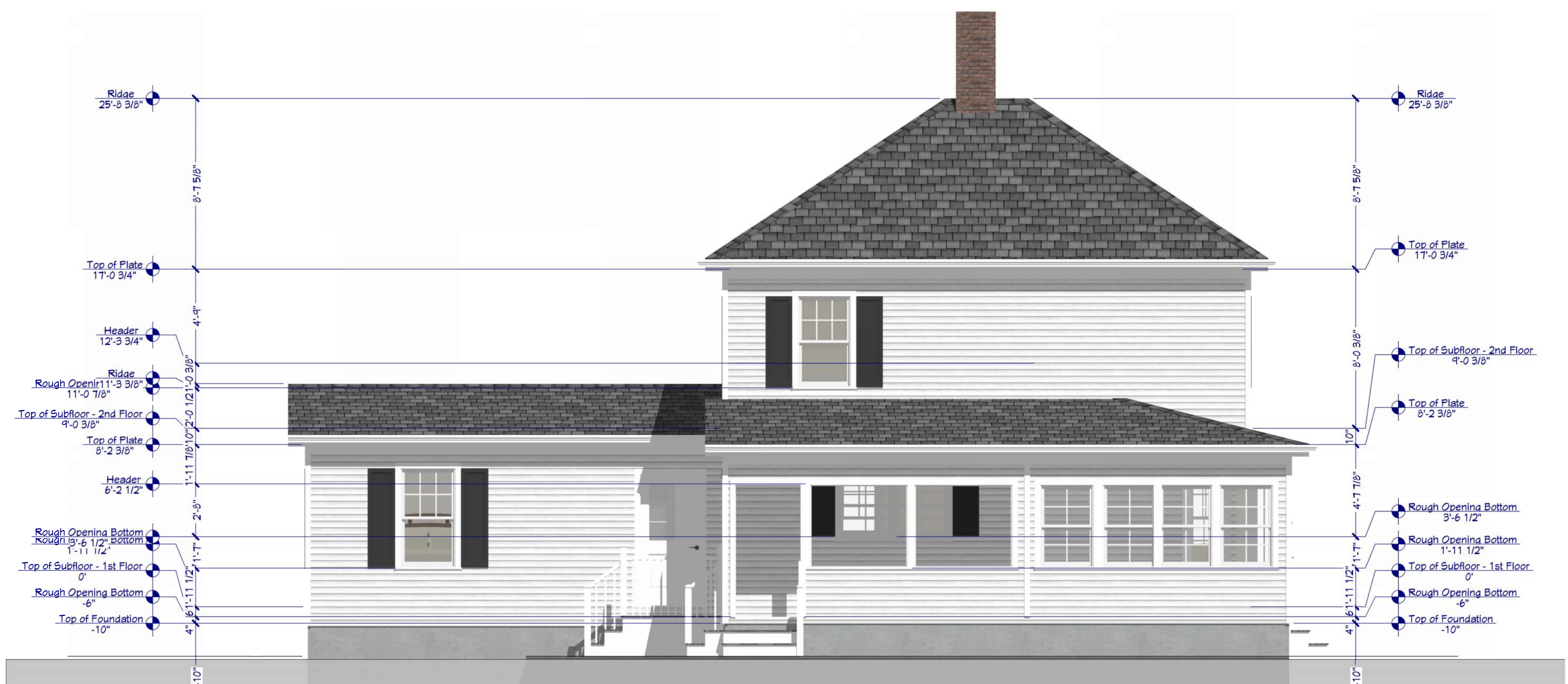
Exterior Elevation Left 1/4 in = 1 ft
