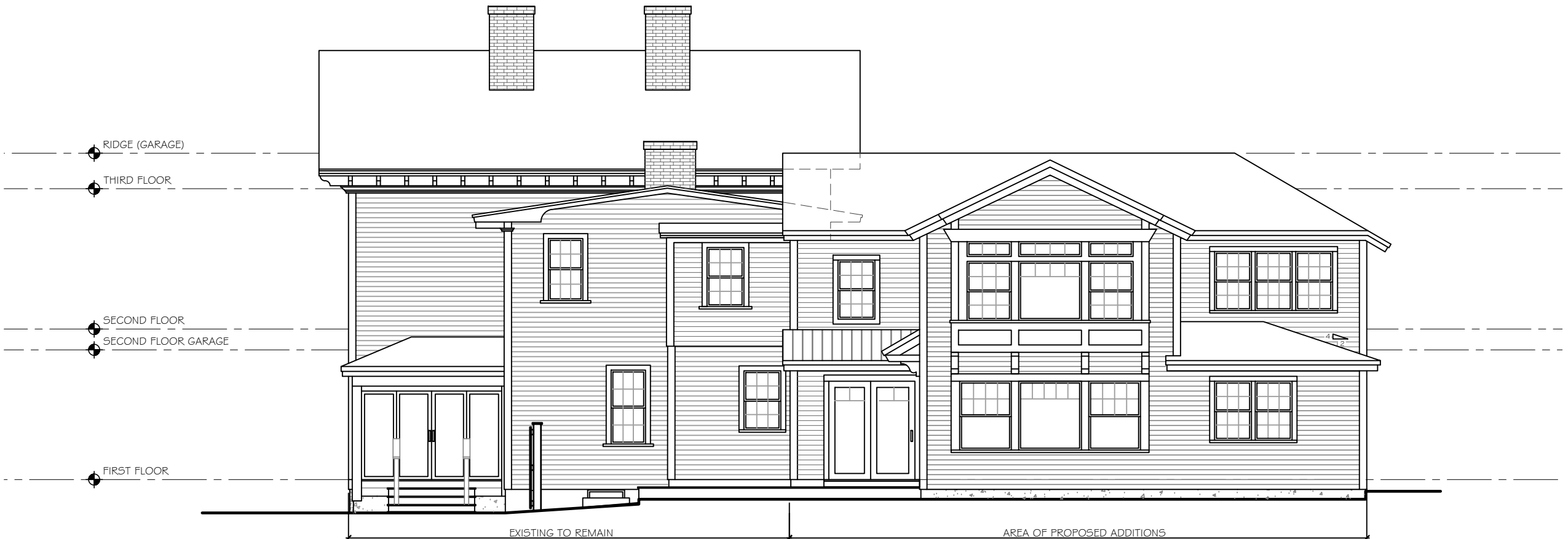
2 PROPOSED REAR ELEVATION
