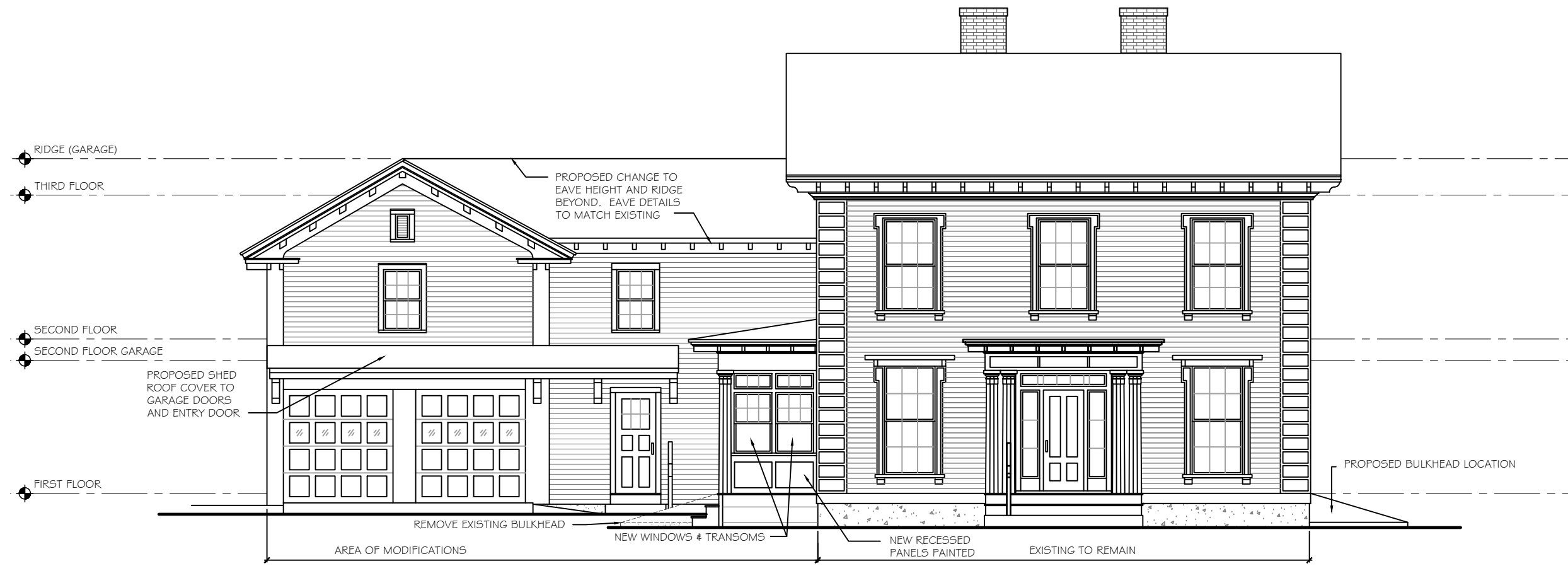
2 PROPOSED FRONT ELEVATION
