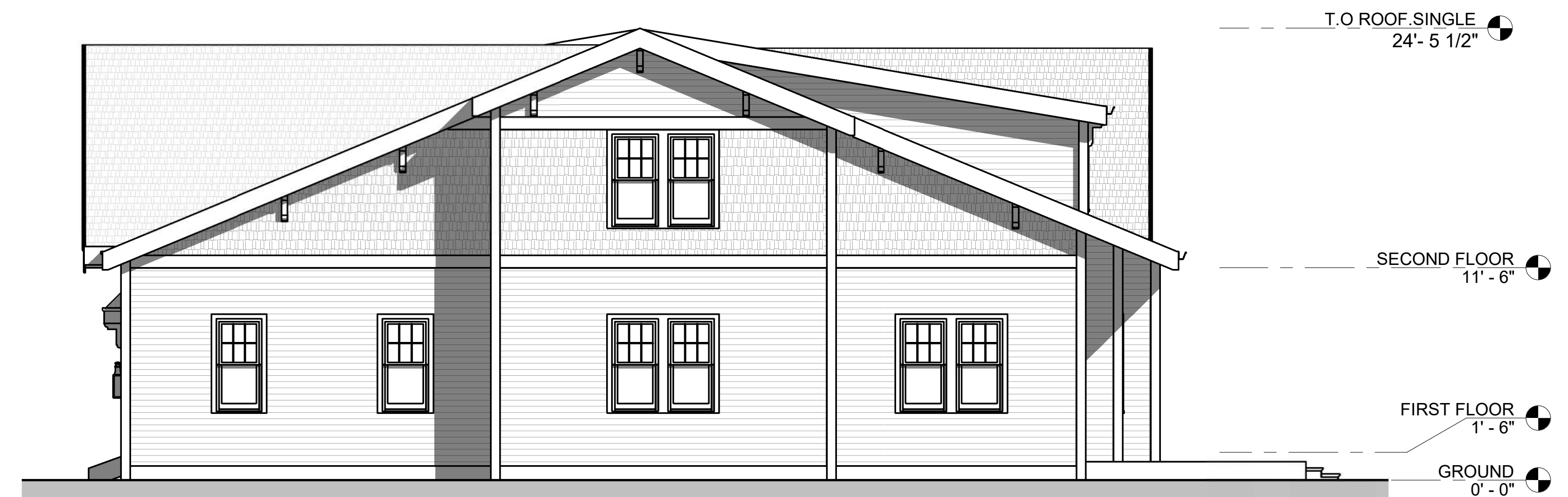
3 SINGLE FAMILY RIGHT ELEVATION 3/16" = 1'-0"
