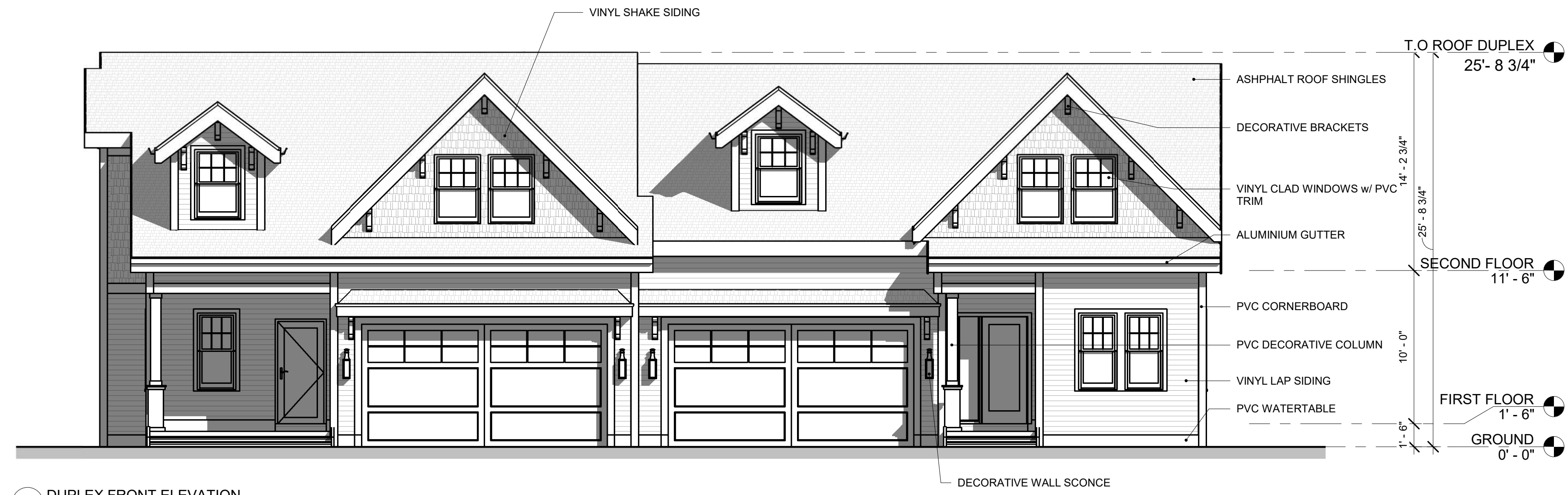
1 DUPLEX FRONT ELEVATION 3/16" = 1'-0"
