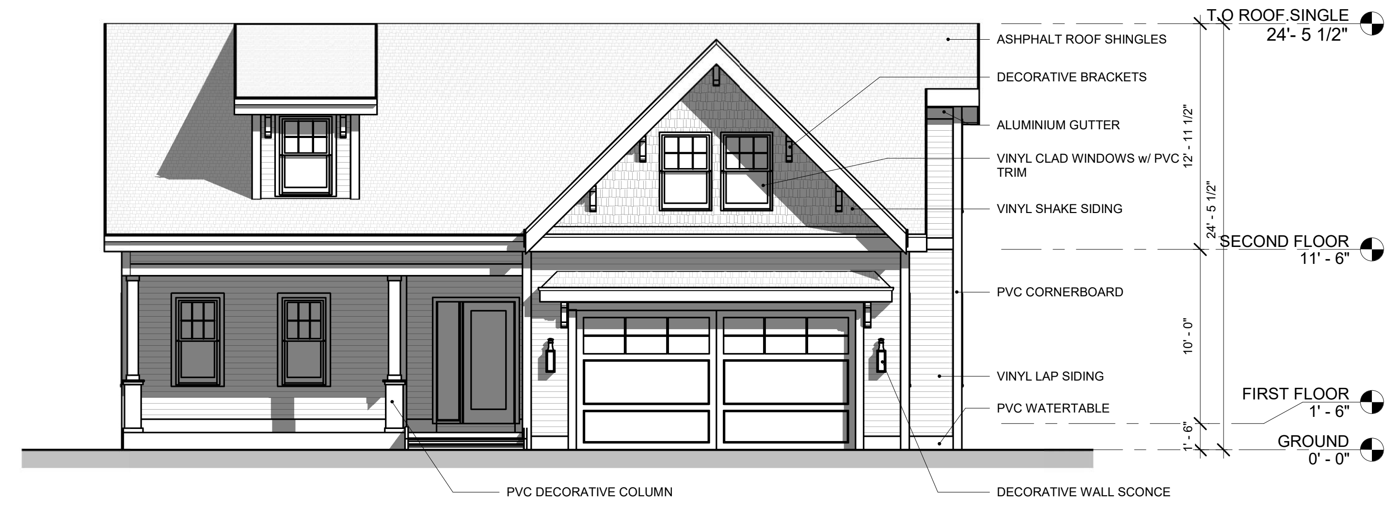
1 SINGLE FAMILY FRONT ELEVATION 3/16" = 1'-0"
