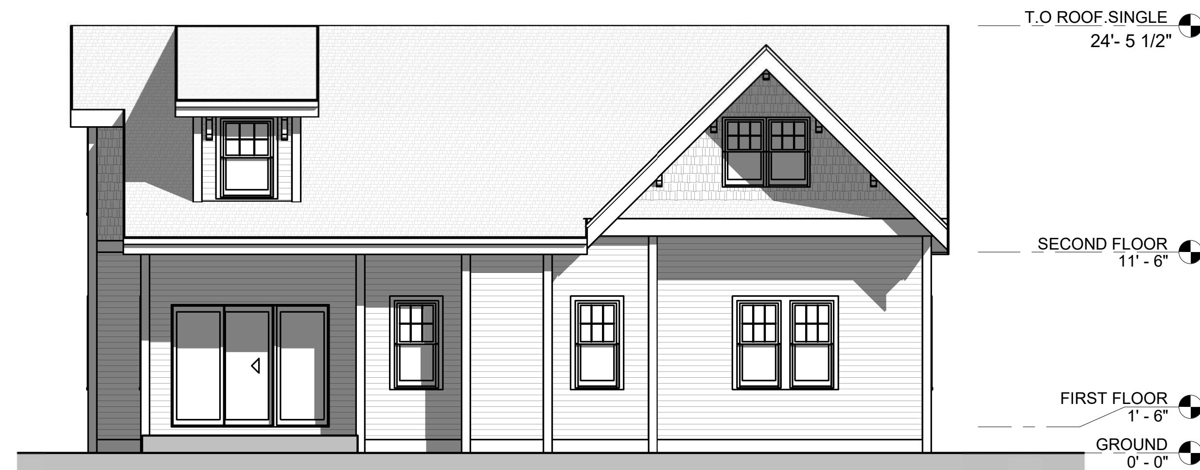
4 SINGLE FAMILY BACK ELEVATION 3/16" = 1'-0"
