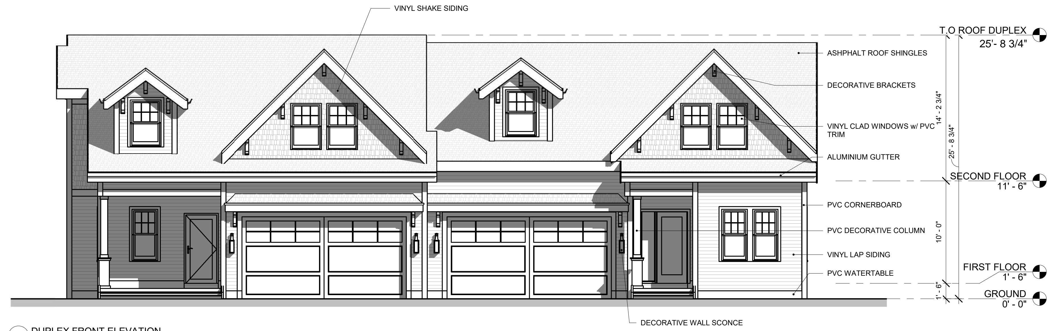
1 DUPLEX FRONT ELEVATION 3/16" = 1'-0"
