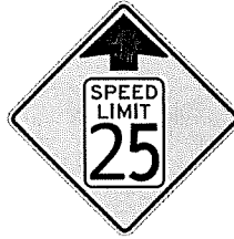
(c) Reduced Speed Limit Ahead (W3-5) sign. Source: MUTCD (edited by staff)
