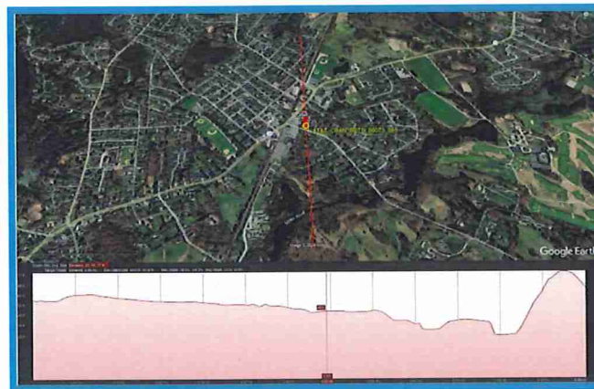
Figure 3b: USGS Elevation Profile Along the North to South Azimuth AT&T Site CRAN_RCTB_00073_665 (Picture courtesy Google Earth ©2024 and may not represent current conditions)
